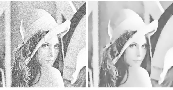
Fig. 2. Isotropic Perona-Malik diffusion (right) is applied to a noisy initial image (left).
